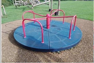
**Finding:** The item is slightly loose in its foundations or the bearings may be worn
